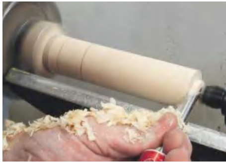
▲ Pic.2 Because I was planning to go very thin, I decided to hold one end in a chuck. About 8mm of timber right at the end is wasted, so I take that down with the 10mm skew chisel
